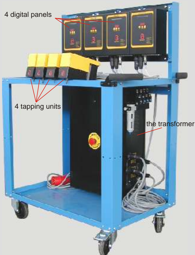
Fig. 1: 4 tapping units with 4 digital panels and the transformer
